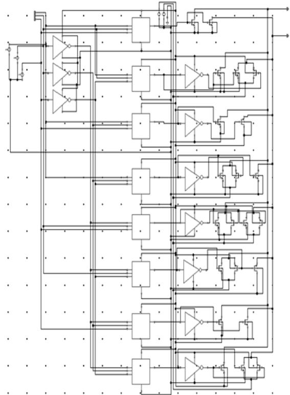
Figure 6: Schematic of Binary to Ternary Converter
